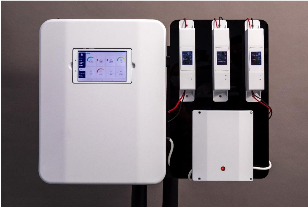
Fig. 1 DC power supply system with SDB
